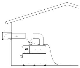
FIG. 22 Sidewall Vent
